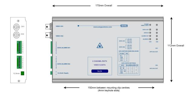
The **AMG5724** is a **DUAL** standalone system which provides two independent channels, each designed to receive one video signal and transmit and receive one bi-directional alarm plus one data signal over one Singlemode optical fibre.
